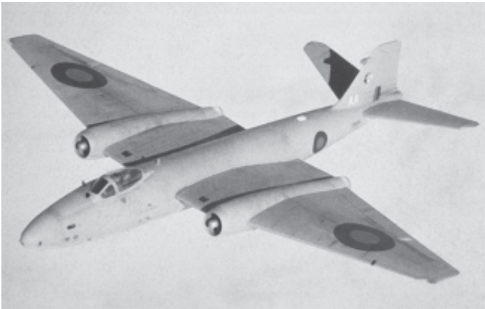
Fig 1-2 Canberra was the first jet bomber to enter RAF service. The PR9 version continues in RAF service as a photographic reconnaissance aircraft.
